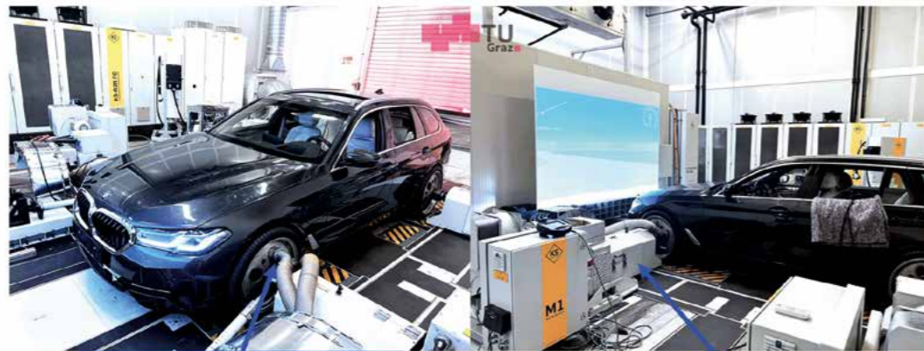
Constant-velocity joint shafts are used instead of the original vehicle wheels
