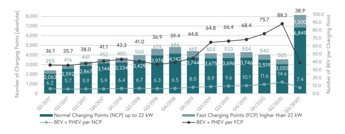
The figure shows publicly available normal and fast charging points according to Directive 2014/94/EU. In total there are 6,849 normal charging points and 1,300 fast charging points until the end of the third quarter of 2020. At this moment there are about seven electric cars (BEV and PHEV) on one NCP and about 39 on a FCP.
